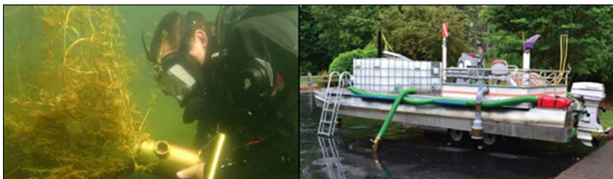
Figure 90: DASH – Feeding EWM into the underwater Suction Hose (Marinette Co.); and a sample DASH Pontoon Boat (Beaver Dam Lake Management District)
