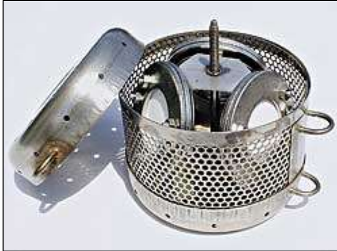
Figure 99: POCIS devices (discs with white centers) shown mounted in a deployment canister. (Source: www.est-lab.com/pocis.php )
