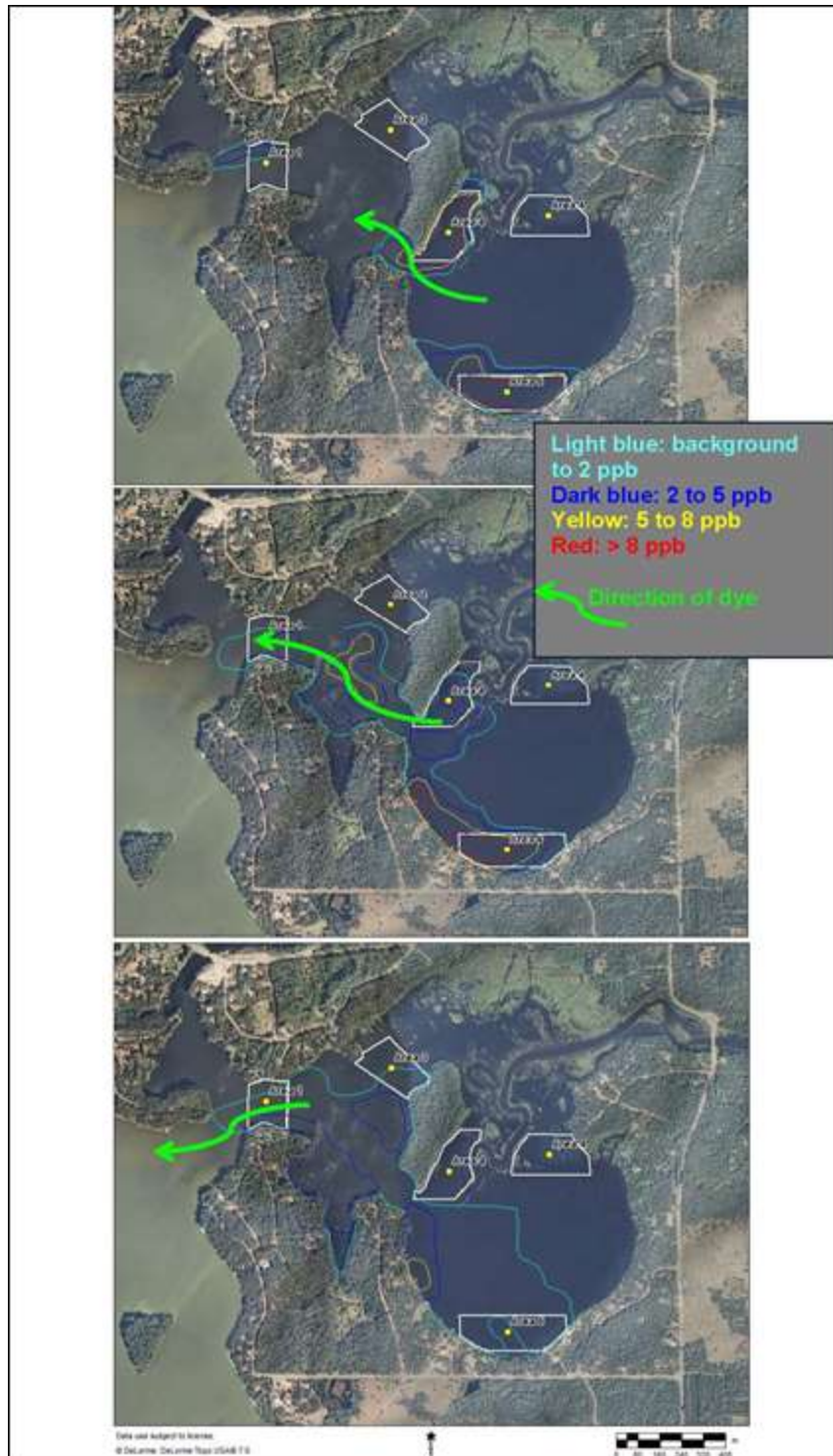
Figure 47: Fall 2014 dye concentration and movement 2, 7, & 27 hours post-dye application
