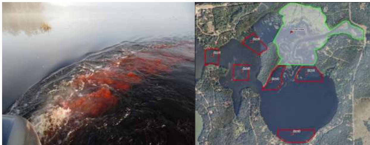
Figure 45: Rhodamine dye applied to waters of the Minong Flowage (left) and the designated study areas (right). The area outlined in green was considered wild rice water for the purposes of the study.
