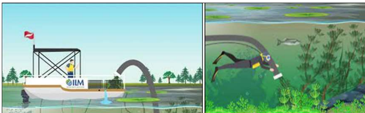
Figure 89: DASH boat and underwater operation (ILM Environments)
