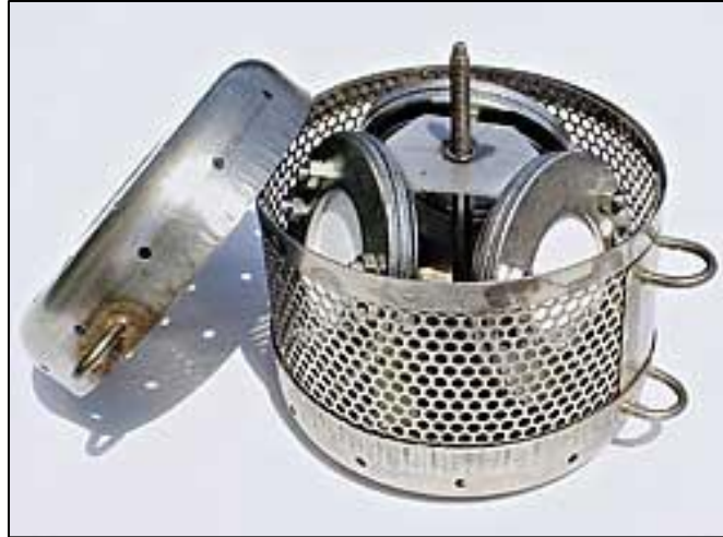
Figure 3: POCIS devices (discs with white centers) shown mounted in a deployment canister. (Source: www.est-lab.com/pocis.php )
