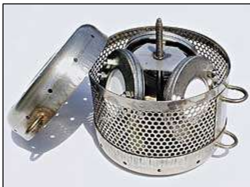
Figure 2. POCIS devices (discs with white centers) shown mounted in a deployment canister. Note: In the figure, three POCIS are mounted, whereas this study deployed one POCIS per canister. (Source: www.est-lab.com/pocis.php )
