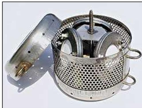
Figure 23: POCIS devices (discs with white centers) shown mounted in a deployment canister (Source: [www.est-lab.com/pocis.php](http://www.est-lab.com/pocis.php))
